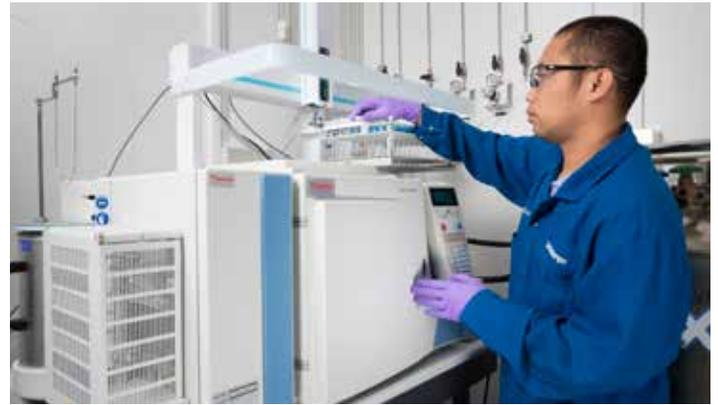
Gas chromatography with isotope-ratio mass spectrometry measures the isotopic composition of compounds in reservoir fluids.
