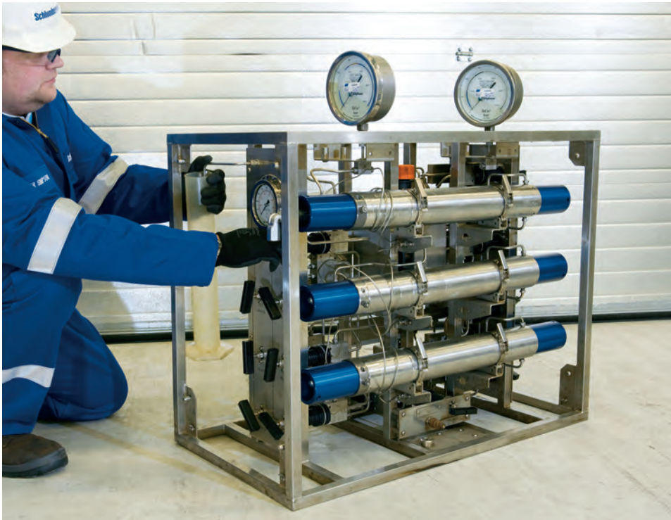
Wellhead sampling manifold.
