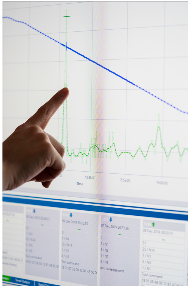
Real-time confirmation of toolstring position by the gamma ray count via Muzic wireless telemetry.
