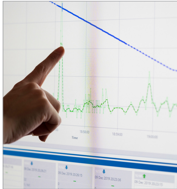
Real-time confirmation of toolstring position by the gamma ray count via Muzic wireless telemetry.
