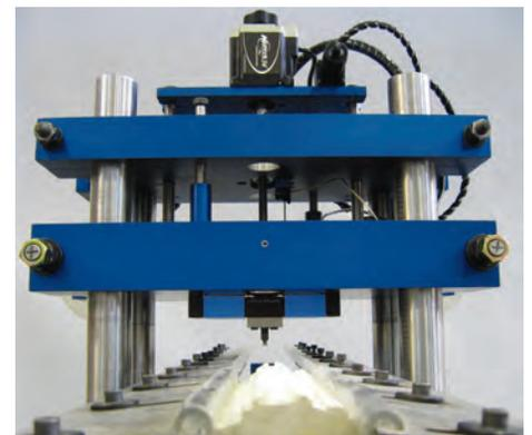
Profiler core scratch test system. Scratch testing is used to help correctly define facies and heterogeneities that would be difficult to discern by geologic description or log characteristics alone.
