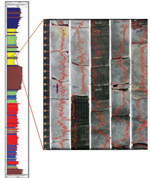
Vertical heterogeneity at log scale. Similar rock class colors represent units with similar material properties. The profile overlaying the colors is the measured continuous core strength, but displayed at lower (log scale) resolution. The insert shows an example of a core section where the transition between carbonate units and an argillaceous mudstone unit is apparent.
