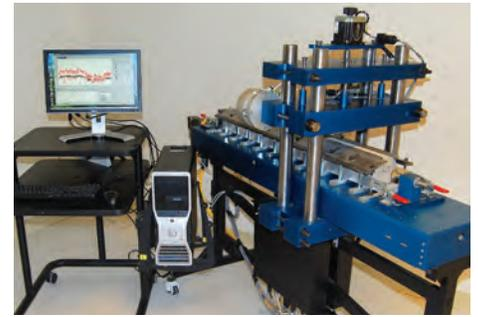
*Core scratch test system and scratch test results on screen. The depth of the scratch on the core's surface indicates rock strength (red curves), which can be correlated to rock mechanical properties.*
