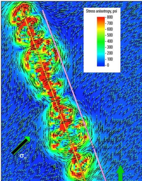
Parent well fracture network with stress anisotropy shown as color in the background (red is high; blue is low). Maximum stress azimuth is shown by black body arrows with green tips. Far-field orientation is NE-SW, but stress rotates around the depleted zone, influencing the hydraulic fracture propagation from the infill well.
