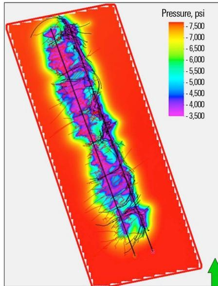
Depletion-induced pressure field simulated for the combined system, including the parent well and infill well. Pressure is shown as color in the background (red is high; purple is low). The fracture network loses connection to the wellbore of the parent well at each stage with fracture hits, which causes faster decline on pressure and production (right).
