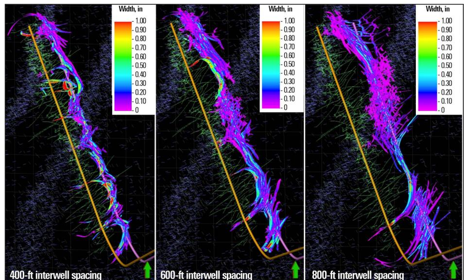
Simulated complex fracture network for the infill well at different interwell spacing from the parent well.
