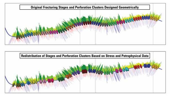
LWD images and stress data helped an independent operating company optimize perforation placement and fracture stages.
