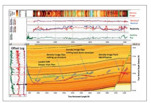
*EcoScope and sonicVISION data revealed dip changes in Eagle Ford layers. The borehole image enabled the identification of a fault near the toe of the lateral.*
