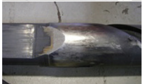
Examples of component damage caused by excessive closing force.
