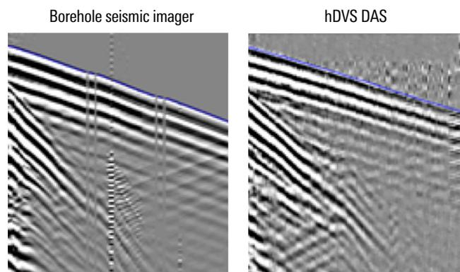
*The hDVS DAS system acquired highly usable checkshot data that matches the conventional borehole seismic survey but with only 10% of the shots required and at a 98% reduction in acquisition time.*
