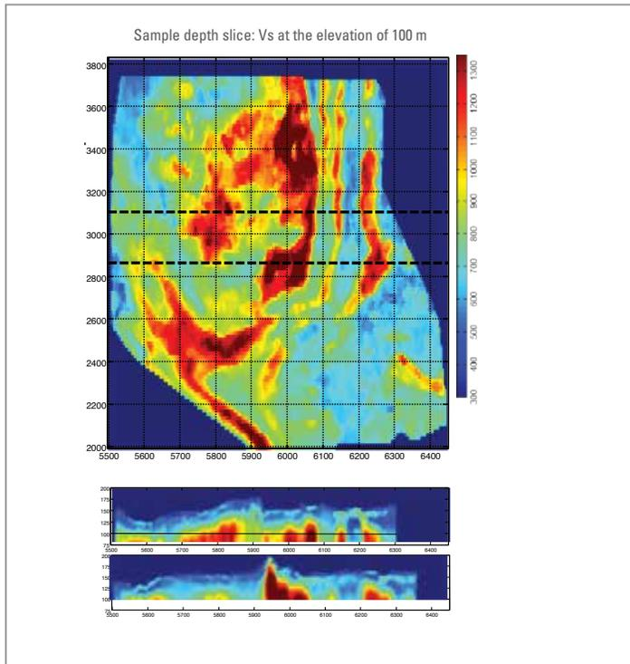
*Broadband point-receivers recorded low-frequency surface wave energy which was used to build an accurate near-surface velocity model using the SWAMI\* surface wave analysis, modeling, and inversion technique.*
