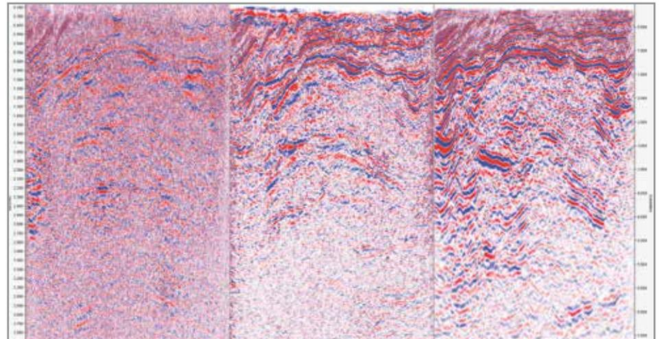
*TTI anisotropic velocity model and depth migration reveal previously unseen structural detail. Brute stack (left). Prestack time migration (center). RTM prestack depth migration (right).*
