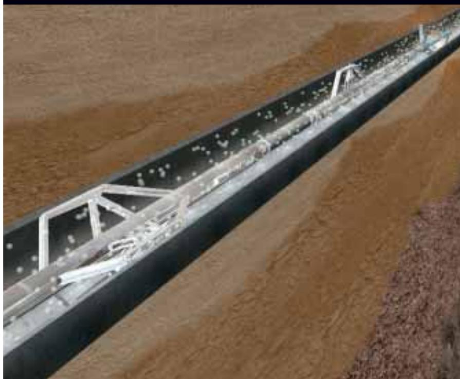
The MaxTRAC design uses gripping cams to minimize wellbore or formation damage and counteract lift forces prevalent in high-flow-rate wells. The cams lock the toolstring in place even when the tool is stationary and high lift forces are trying to carry the tool and cable uphole.
