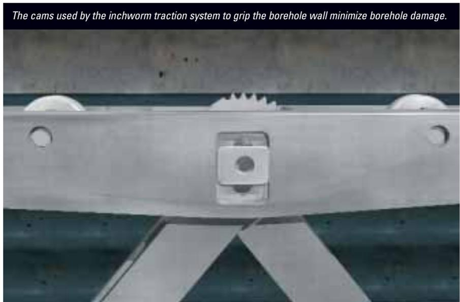
The cams used by the inchworm traction system to grip the borehole wall minimize borehole damage.
