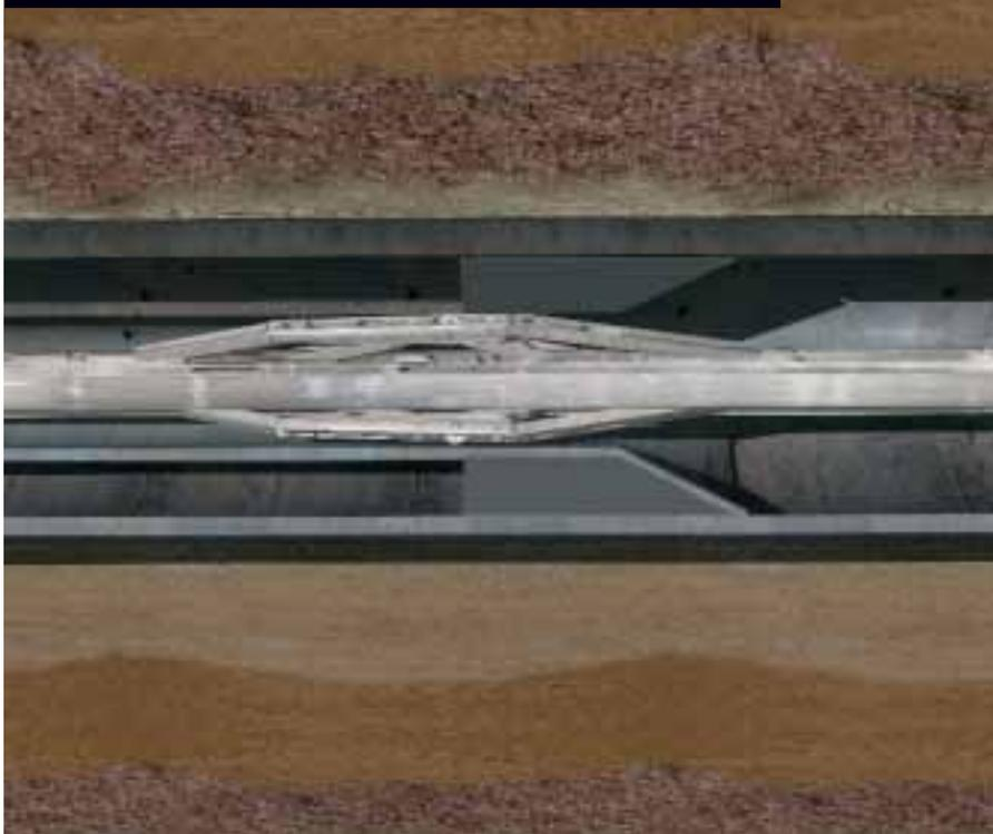
*Washouts can be addressed by adding tractor sections; any two with good wall contact will drive the MaxTRAC system.*
