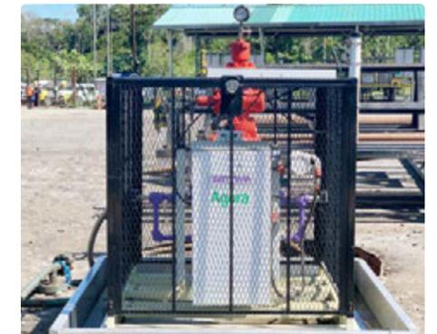
*The solar-powered AgoraGateway ruggedized edge computing solution collects, integrates, and transmits data from any field device, significantly reducing trips to the wellsite.*
