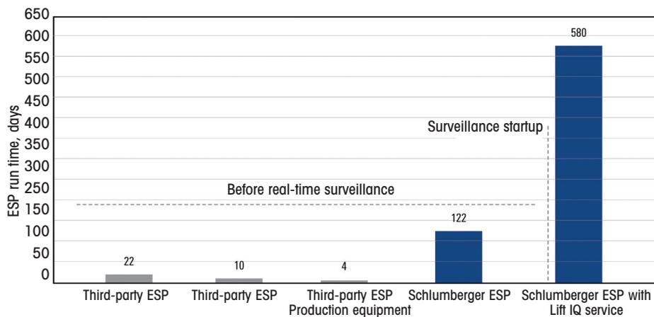
**FIGURE 1. Real-time surveillance helped Bahar Energy substantially improve ESP runlife without installing additional completions equipment in an offshore well in the Gum Deniz Field.**
