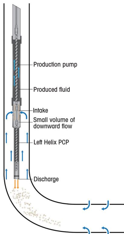
**FIGURE 2. The Left Helix pump design incorporates a bottom rotor to pump a small percentage of fluid downward, which prevents sand accumulation at the intake. The design also replaces the conventional bottom tag with a top tag to reduce plugging risks. (Source: Schlumberger)**
