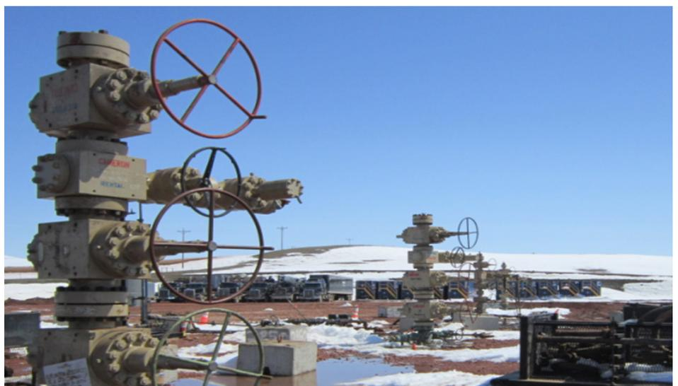
*Cameron frac trees on the operator's Golden Creek/Burner pad in the Bakken Shale.*
