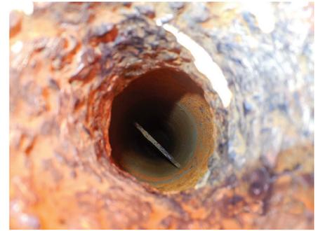
**Fig. 4.** The milling shoe after being pulled out of hole without inner bar.
