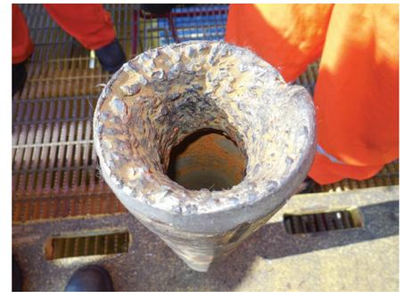
and began the recovery process. After a total of 43 runs over 20 days, the 9,977-ft CT pipe was recovered to the surface, with the CT weight gradually increasing from 0 to 39,000 lbf, Fig. 5.
