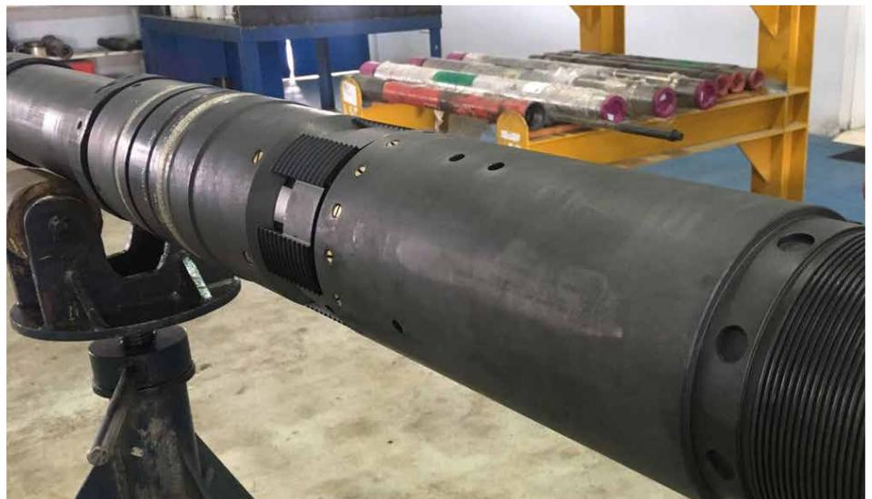
*The first thermal COLOSSUS liner hanger systems manufactured in Oman are designed to withstand superheated steam at 600 degF and prolonged acid exposure.*
