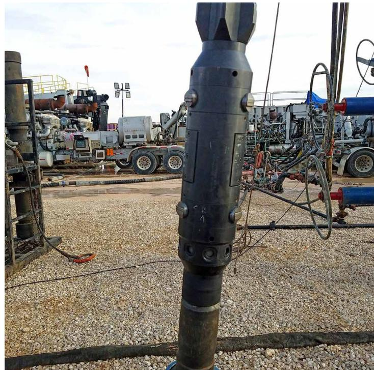
*Schlumberger reclosable CT frac sleeves reduced rig-up and rig-down times as well as the time between stages. In addition, they provided the flexibility for rigless zonal shutoff (e.g., for sand management) later in the life of the well.*
