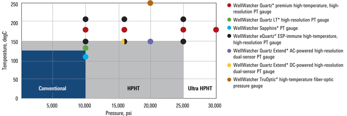
The graph shows the environmental applications in which WellWatcher system downhole gauges are most appropriate. The WellWatcher eQuartz gauge is suitable for temperatures as high as 200 degC and pressures as high as 25,000 psi.
