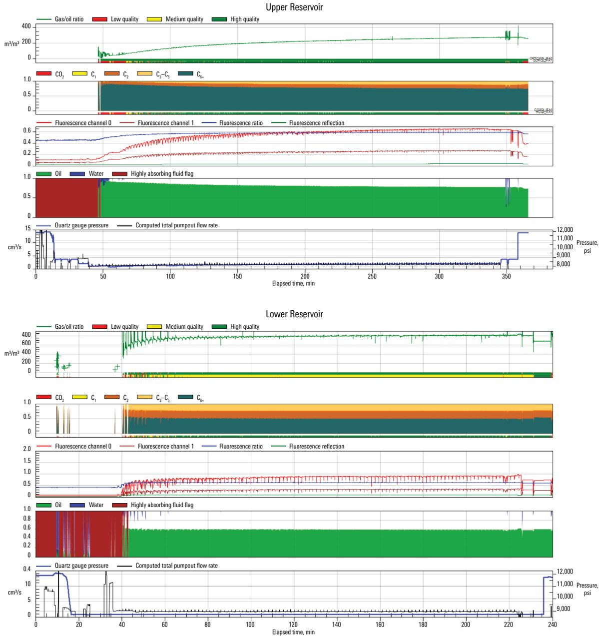
Real-time DFA conducted with the MDT Forte-HT tester and 5-in Saturn probe at stations in the upper and lower sections of the reservoir document the difference in composition within the hydrocarbon column.
