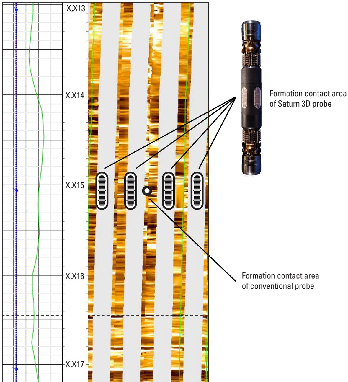
High-quality borehole images obtained with the OBMI oil-based microimager were used to identify areas for investigation, first with conventional probes and then with the Saturn 3D radial probe. It was not possible to perform pressure measurements with the small contact area of the conventional probe. Pressure measurements and fluid samples were obtained with the Saturn radial probe and its large 79-in<sup>2</sup> contact area.
