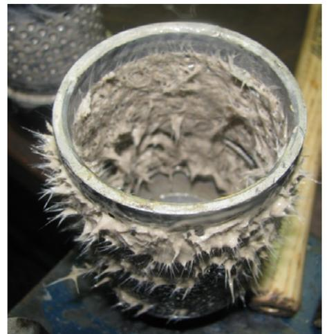
*The FORM-A-BLOK AS pill forms a plug while defluidizing through porous formations, preventing losses.*
