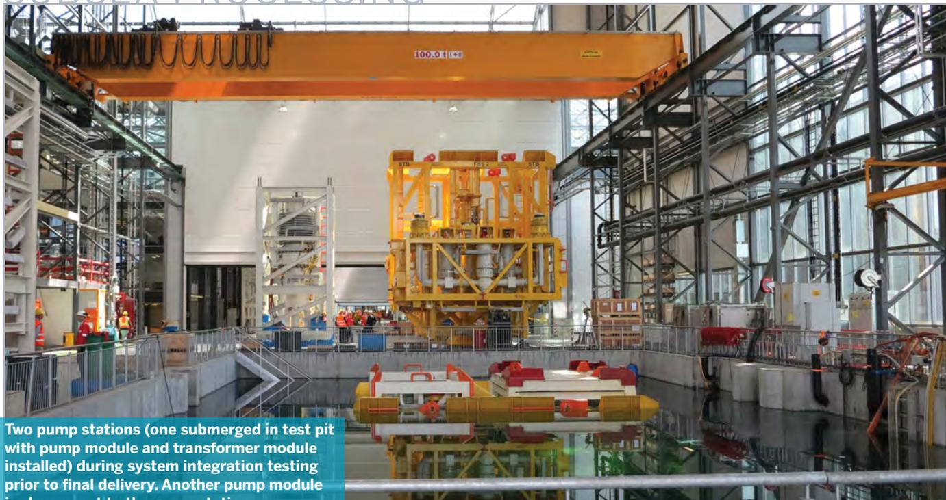
Two pump stations (one submerged in test pit with pump module and transformer module installed) during system integration testing prior to final delivery. Another pump module is shown next to the pump station.
