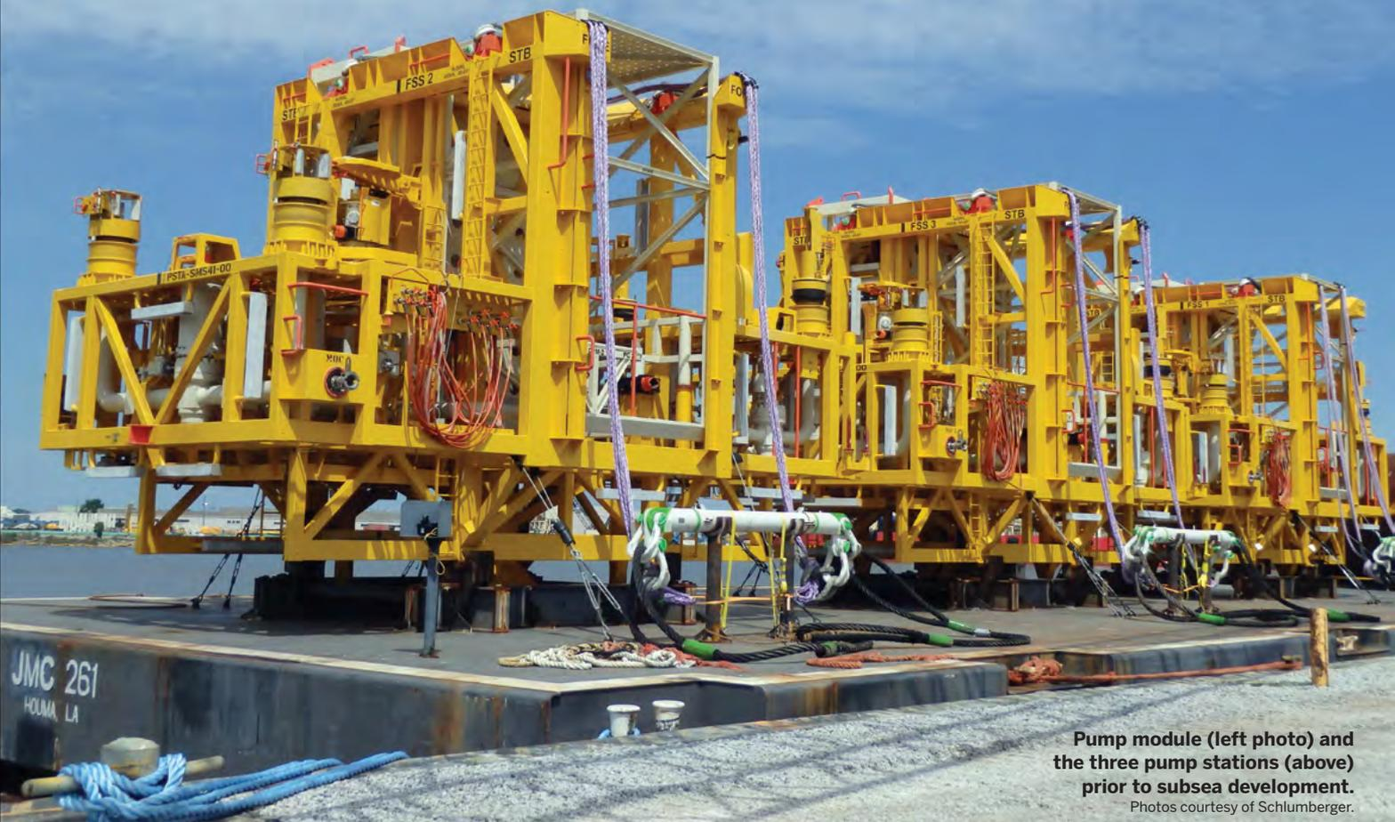
**Pump module (left photo) and the three pump stations (above) prior to subsea development.**
