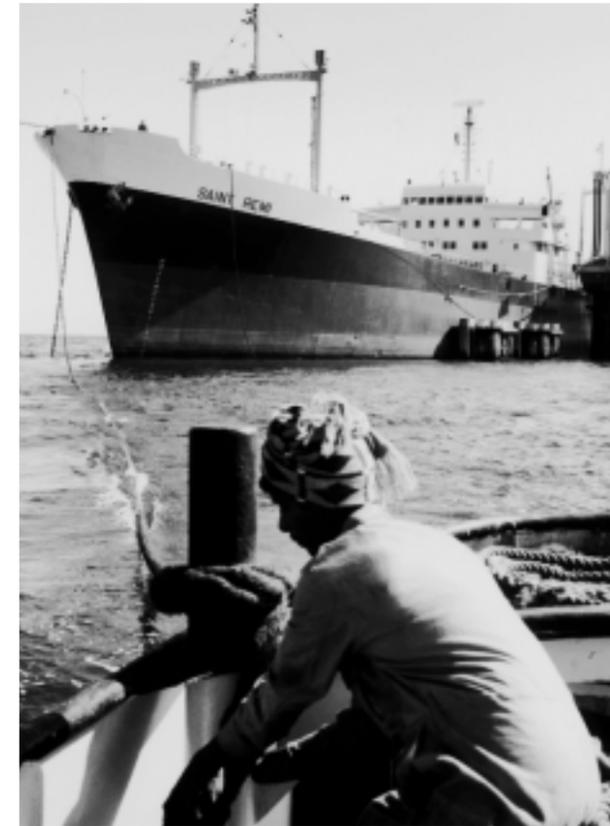
Figure 16.8: Das Island tanker terminal. French tanker Saint Remi being moored at the terminal. A head line is being taken on board a work boat
