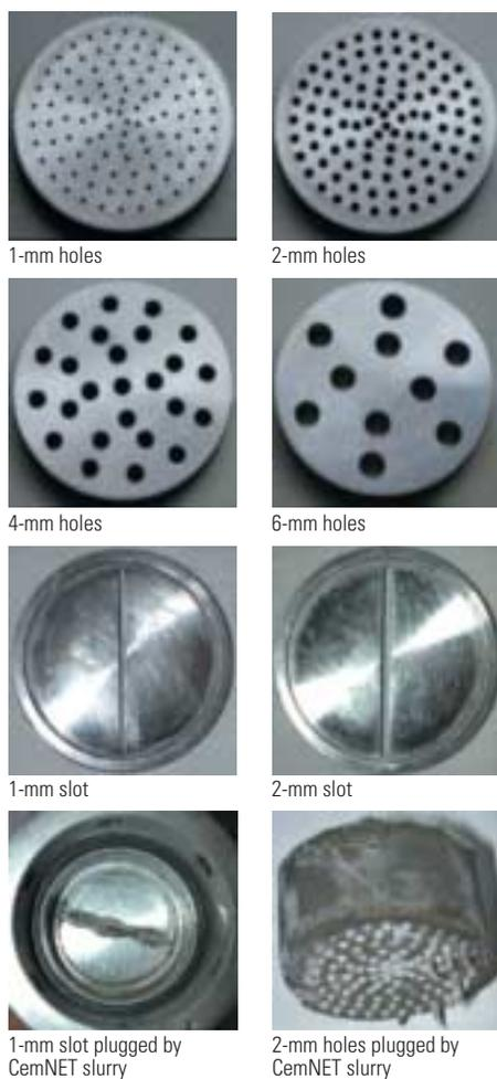
▲ Laboratory testing of fibrous slurries. An API fluid-loss cell was modified to test CemNET slurries (top). The top of the test cell acts like a piston; the plate at the bottom simulates a loss zone. Round holes in the plates, measuring 1, 2, 4 and 6 mm [0.04, 0.08, 0.16 and 0.24 in.] in diameter, simulate high-permeability zones; the slotted plates represent fractures 1 and 2 mm wide (middle). After testing, the plates with slots or holes are plugged with fibrous slurry (bottom).
