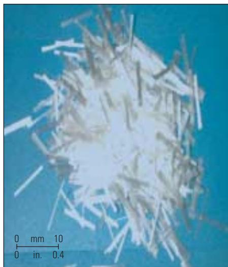
^ CemNET technology. Dry CemNET fibers are easy to handle (left). Once mixed with water, the fibers form a mat-like network across zones of lost circulation (right).
