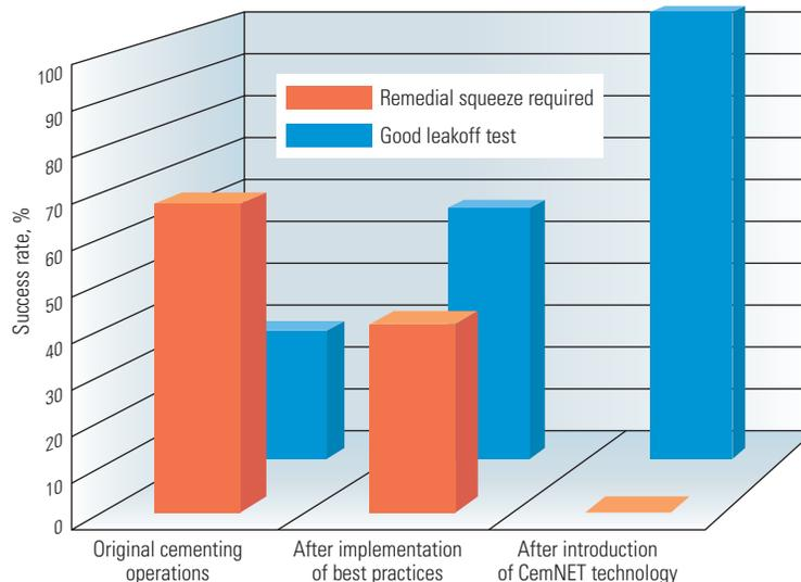
^ Cementing success rates using typical cementing techniques, best practices and CemNET technology in the Tampen area. Red bars indicate subsequent need for remedial cementing; blue bars indicate good leakoff test (LOT) results.
