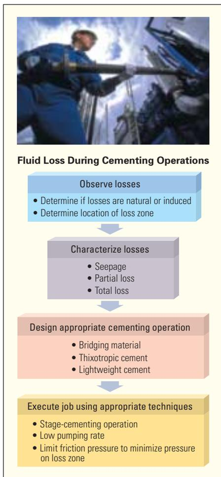
^ Workflow for countering lost circulation during cementing operations.
