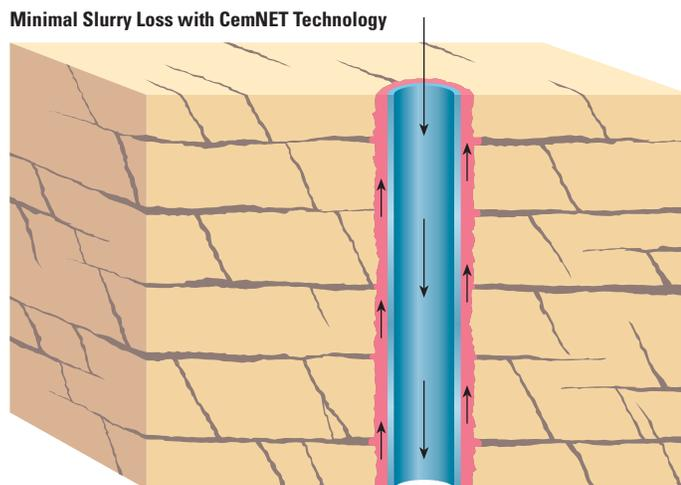
▲ Net-like fibers to bridge loss zones. Fluid loss in fractured formations, shown schematically in red, is an undesirable occurrence during cementing operations (*top*). By adding fibers to cement slurry, a fibrous net forms, the cement slurry builds a filter cake and slurry circulates up the annulus to provide zonal isolation and prevent additional fluid losses (*bottom*).
