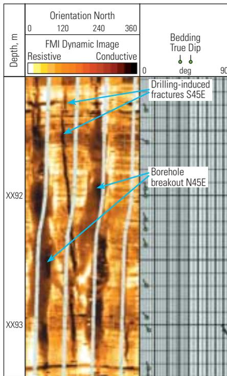
^ In-situ stress direction from borehole images. Borehole imaging data provide detailed stress-direction information (*right*). For example, in a vertical well, borehole breakouts typically are oriented along the minimum horizontal stress direction, while drilling-induced fractures are aligned with the maximum horizontal stress direction (*left*). Induced fractures frequently are near-vertical because the minimum stress is usually horizontal.
