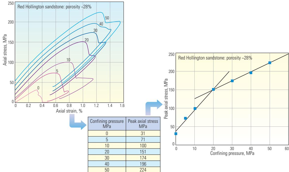
^ Constructing a failure envelope. Reservoir rocks are tested in the laboratory to acquire axial stress and strain data at different confining pressures (top left). Normally, each confining pressure used during testing is plotted against the peak axial stress that occurs before failure (right), allowing the internal friction angle to be estimated.
