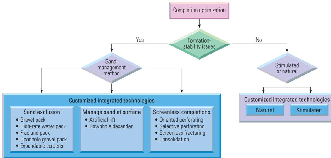
^ Completion options to balance sand control with production requirements. If formation-stability concerns exist, operators can choose between downhole sand-exclusion technologies or screenless-completion methods. They may also choose to manage existing sand production by careful selection of artificial-lift techniques and practices.
