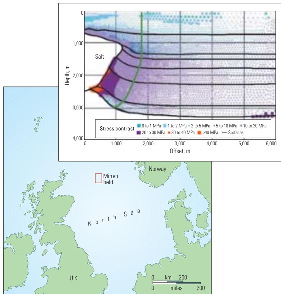
^ Location of Mirren field (*bottom*). Complex stresses surround a salt diapir in Mirren field and must be considered in both drilling and completion operations (*top*). 3D modeling predicts that the maximum stress orientation near the diapir is tilted 20° to 40° from horizontal, making perforated completion design more complex.
