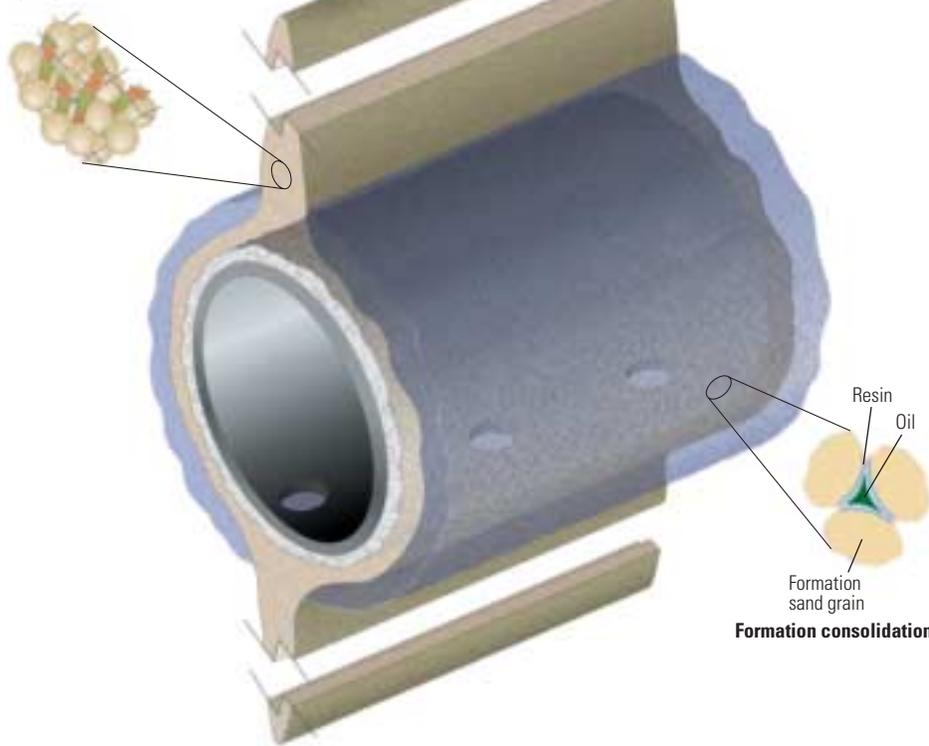
^ Screenless hydraulic fracturing for sand control. A combination of technologies is used to create a stable propped fracture that provides sand control with minimal proppant flowback. The perforating job was designed to optimize the creation of the fracture. After perforating, injected resin was used to consolidate the formation around the wellbore. A TSO fracture created a tightly packed fracture capable of providing sand control and limiting proppant flowback.
