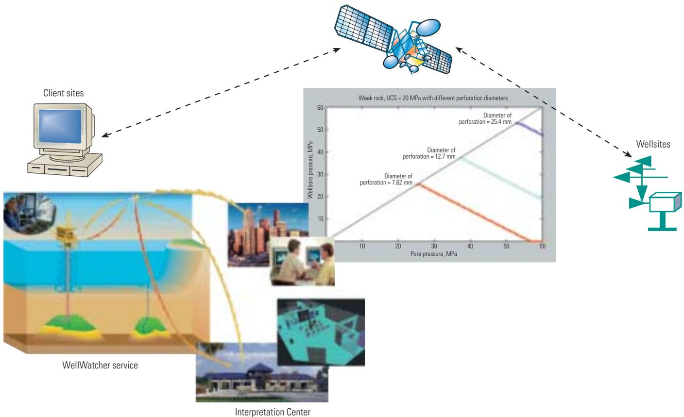
^ Real-time monitoring and control. The negative effects of producing sand and the impact of sand-control efforts can be observed by various downhole and surface measurements. In today's connected oil field, massive amounts of data can be transmitted and sent directly to asset teams and Schlumberger experts for interpretation. The data can be used to update and verify sand-prediction models and reservoir simulators, and to facilitate complete and real-time production optimization.
