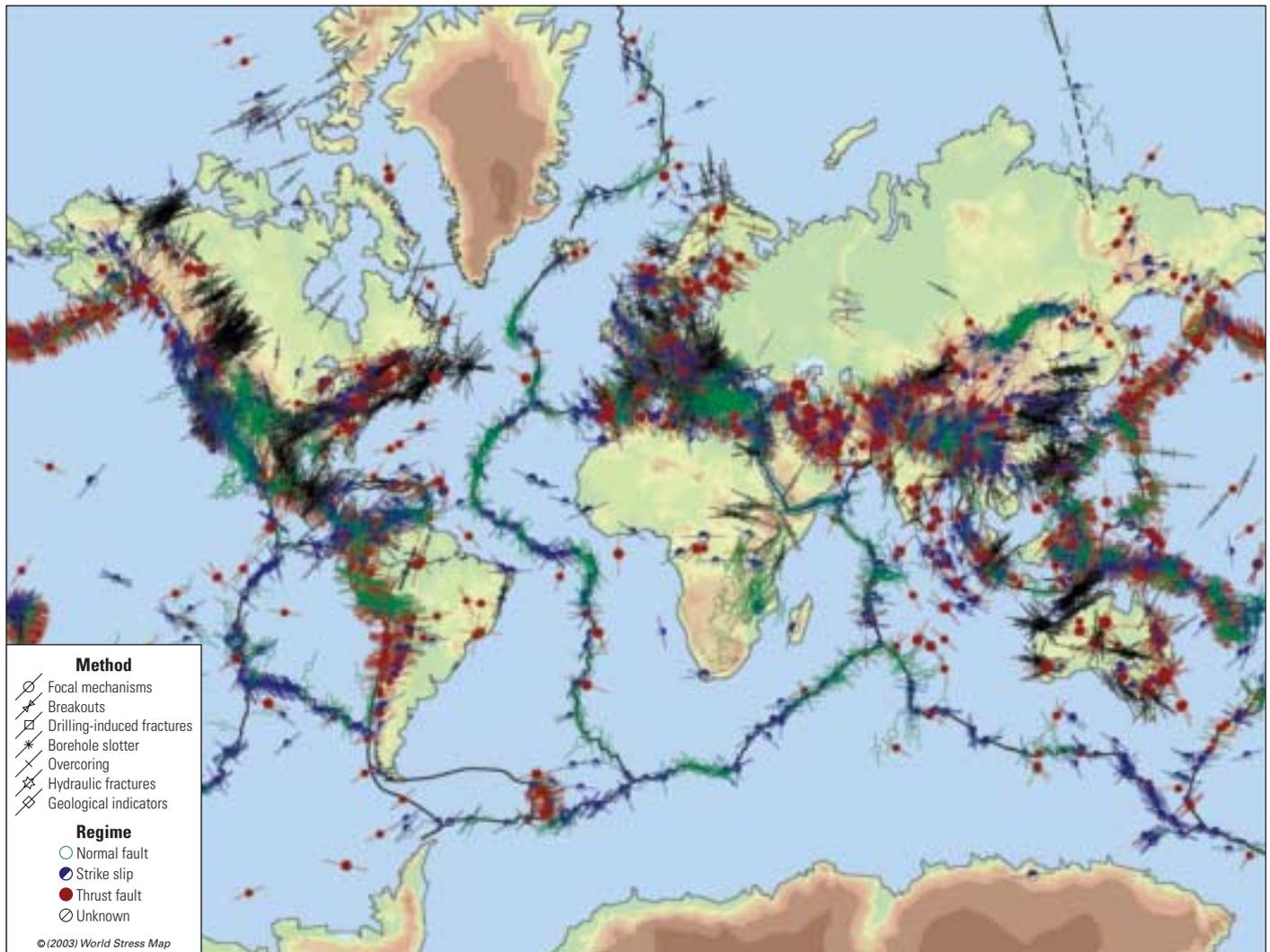
^ World stress map. Stress data are compiled from a variety of sources and displayed on stress maps. Downhole measurements, such as borehole breakout and induced-fracture data, are an important source of this stress information. Hydraulic-fracturing data are also useful but often contain no stress orientation details.
