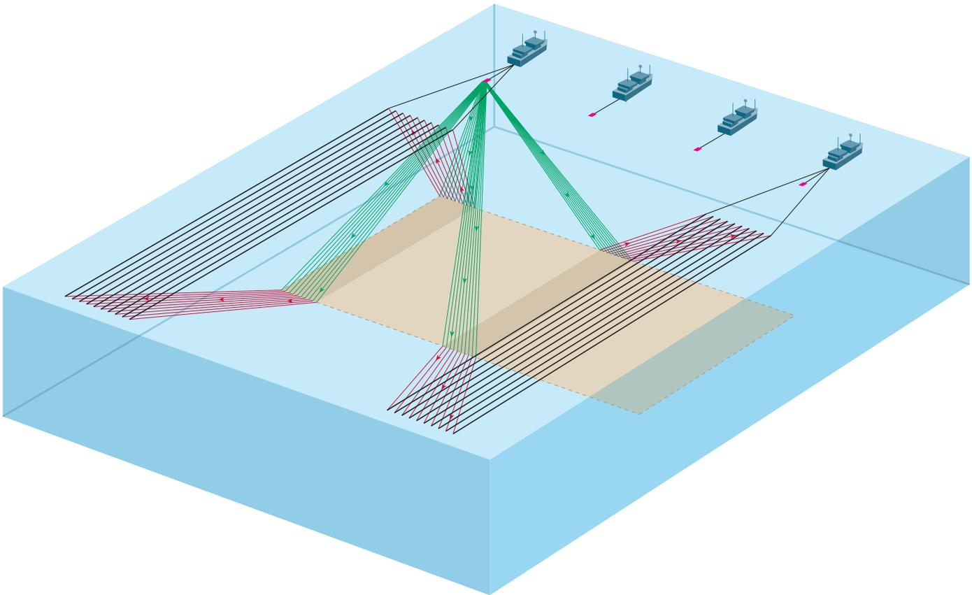
^ A four-vessel wide-azimuth acquisition configuration. Two recording vessels (*left and right*), both equipped with an airgun source array and 10 streamers, are joined by two source vessels (*center*). The source on the left-hand vessel is fired, and data are recorded by streamers on both recording vessels, providing two areas of subsurface coverage (dark tan).
