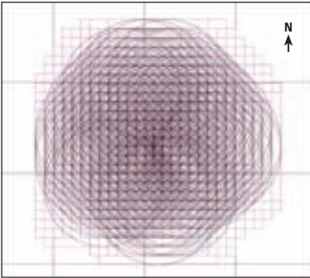
^ Planned source positions for the Tulip survey. The survey plan required the vessel to sail along 145 circles covering the survey area.
