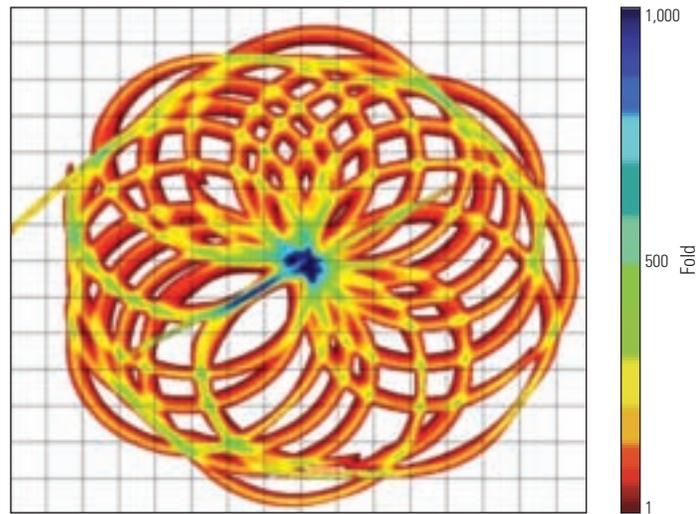
▲ Heidrun acquisition geometry. The test data were acquired as 18 intersecting coils plus one straight line oriented at a heading of approximately 60°. The number of traces (fold) mapping within 25- x 25-m bins is color-coded. Fold rises where circles intersect and is highest in the center of the survey.
