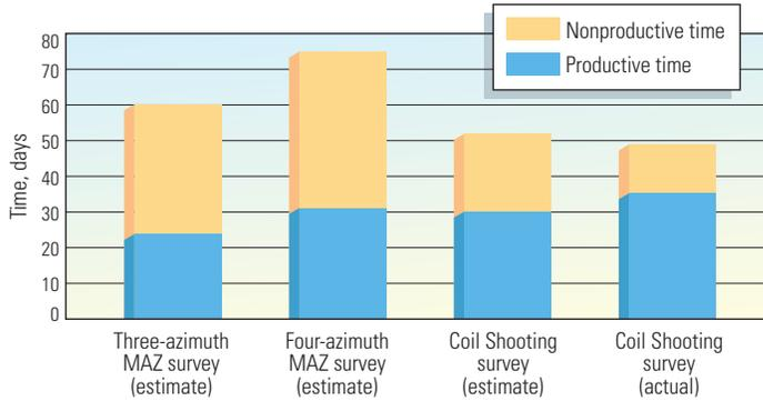
▲ Comparison of acquisition duration for three single-vessel geometries considered for the Tulip survey. The Coil Shooting survey (right) was completed more quickly than was predicted, and more quickly than estimates for MAZ surveys using either a three- or four-azimuth parallel-line geometry.
