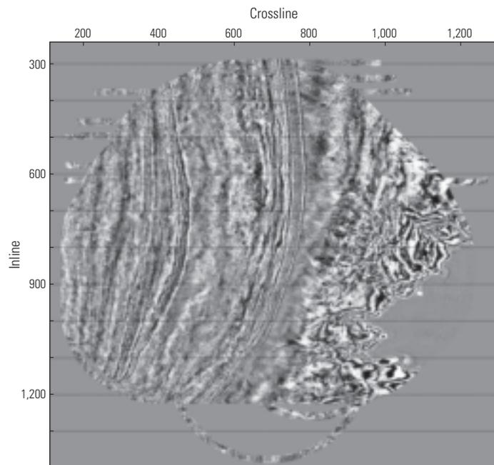
^ Onboard quality-control (QC) displays for the Tulip survey. The example "pie bin" stack section (top), produced during acquisition of one circle, is continuous: if rolled on a cylinder, the start and end of the section will match. The time slice at 2 s (bottom) was extracted from the 3D QC stack volume built onboard during acquisition. This display was made after about 90% of the programmed circles were acquired.
