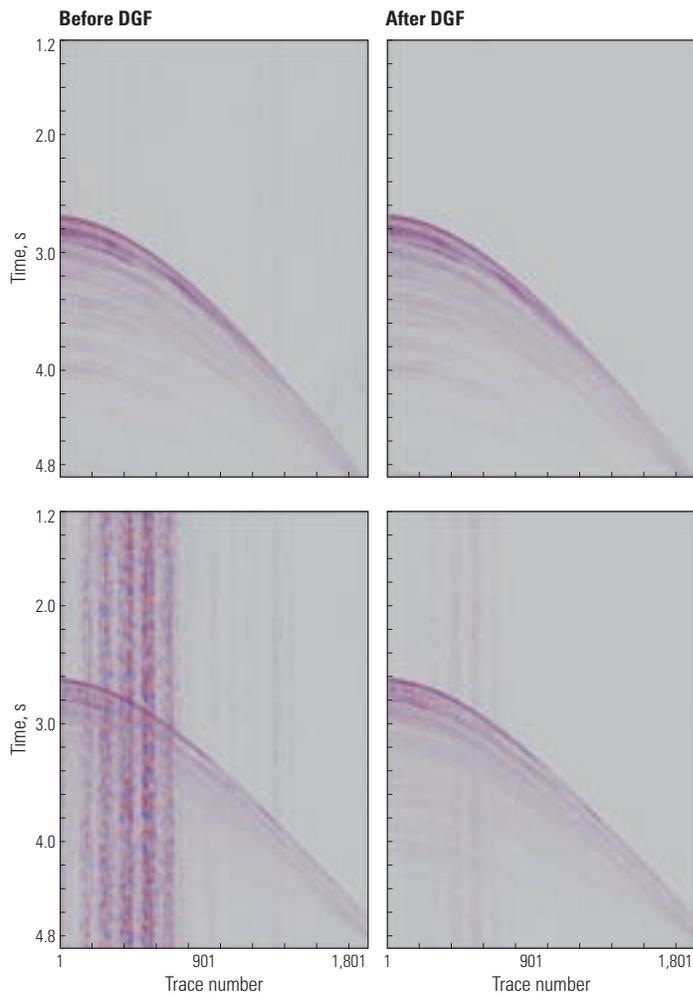
▲ Kozlu field data. At top left is a shot record with low levels of noise. At bottom left is a shot record showing high levels of noise. The first curved line below 2.6 s on the near (left-hand) trace is the water-bottom reflection. In a perfectly noise-free environment, amplitudes above this would be zero. On the right are the same two shot records after digital group forming (DGF), which greatly attenuates the noise. Further noise reduction is achieved during subsequent processing stages.
