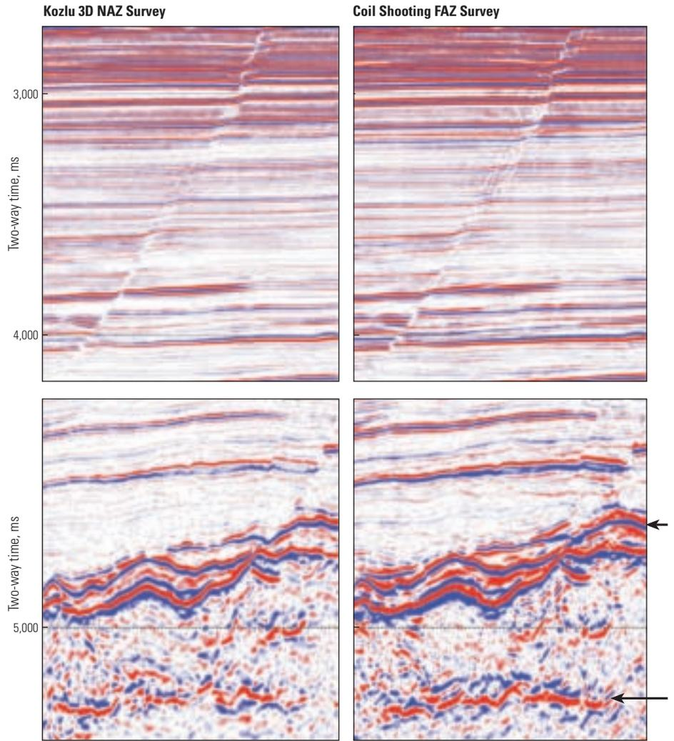
▲ Comparison between NAZ 3D survey (left) and Coil Shooting test results (right). The top comparison shows better imaging of faults in the shallow section of the Coil Shooting data. The bottom comparison displays improved continuity and more detail at the top and base of the reservoir (black arrows) in the Coil Shooting data.
