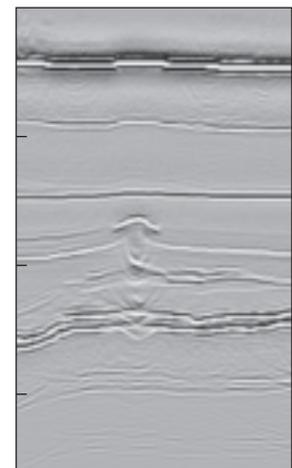
▲ Heidrun modeling results. The depth-velocity model (top) displays the faulted reservoir, coal markers and a small salt body. In the lower panels, the synthetic seismogram (far left) shows the 1D zero-offset reflectivity convolved with the wavelet for the middle part of the model. It represents the simplest seismic response. Note the pull-up of events below the salt body, caused by the high P-wave velocity in the salt. This pull-up
