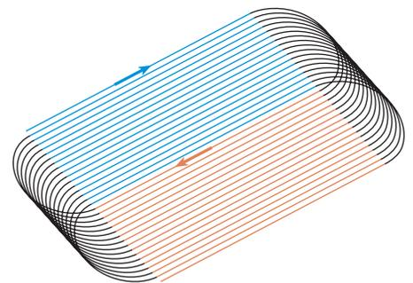
^ Typical conventional deepwater 3D acquisition configuration. The acquisition path follows a straight line (blue arrow) then turns 180° to acquire data in the opposite direction (orange arrow). No data are normally recorded during line turns (black).
