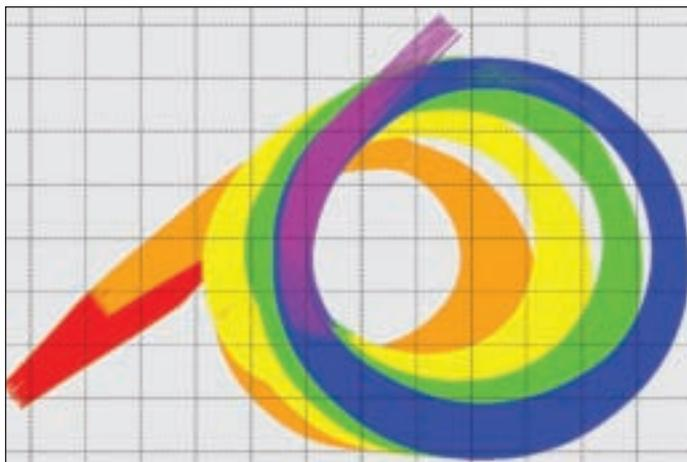
^ Acquisition geometry for the Gulf of Mexico Coil Shooting test. The plot shows areas containing traces from each of four circles acquired with different radii, colored orange, yellow, green and blue.
