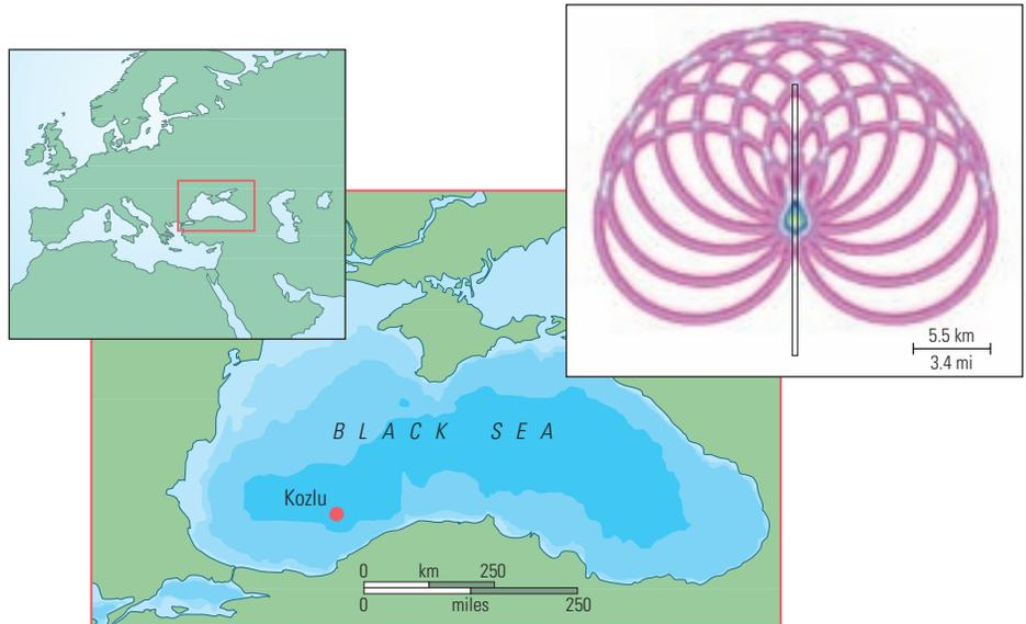
^ Location and design of the Kozlu Coil Shooting test. The Kozlu survey area is in Turkish waters in the southwestern part of the Black Sea. The test data were acquired as a set of nine intersecting circles in a "half-dahlia" pattern (*top right*).
