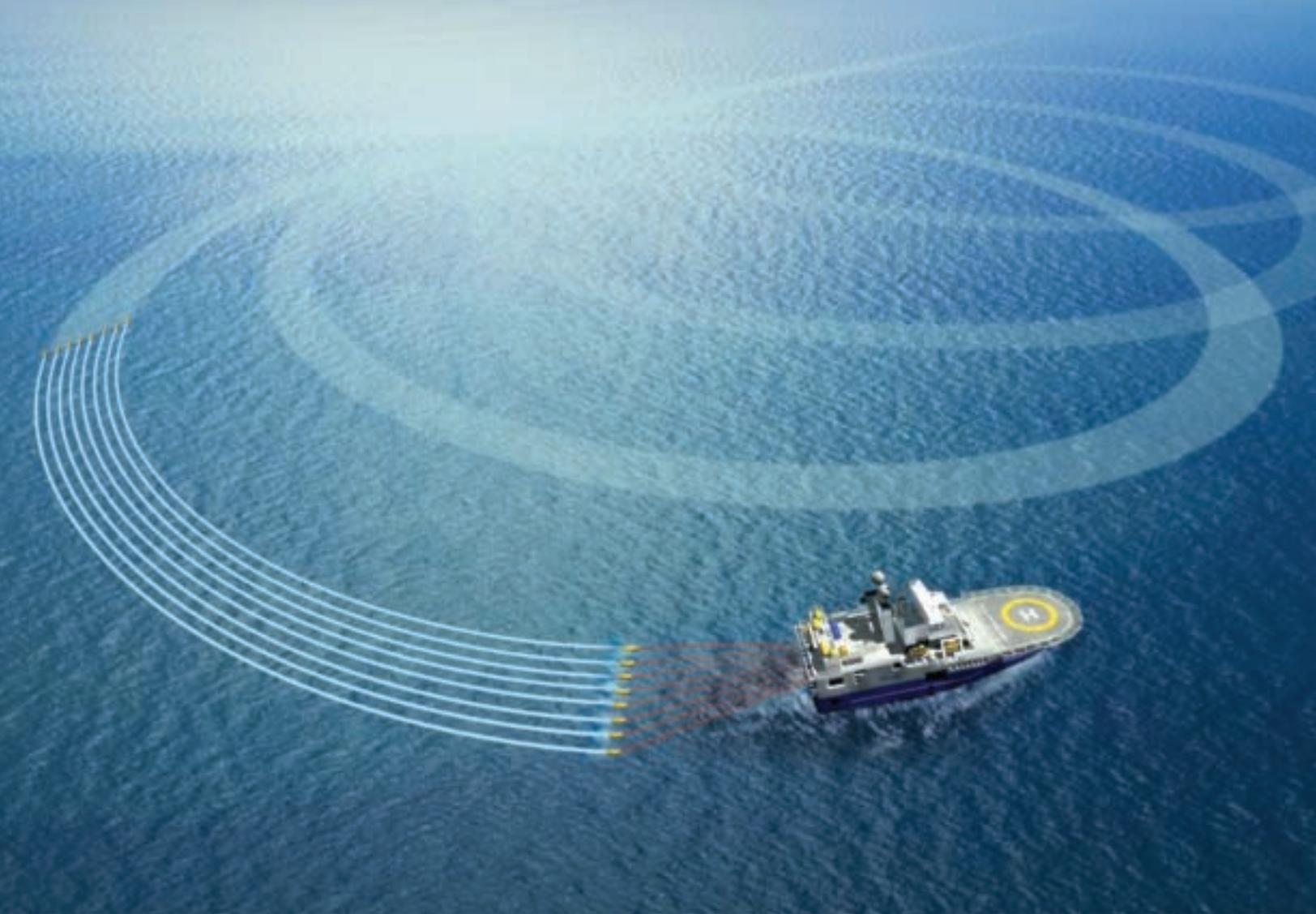
using a single vessel shooting continuously with a circular or curved path. We describe modeling and feasibility tests, which indicate that the technique has considerable potential for efficiently addressing imaging challenges in complex geological settings. Also presented are some details of the world's first full Coil Shooting project.
