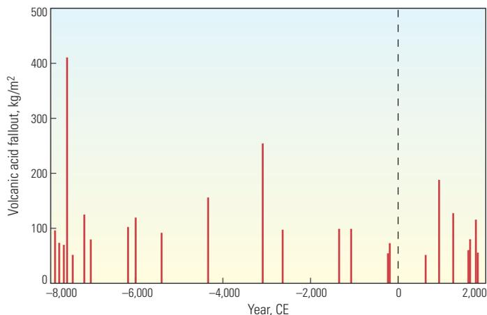
Electrical stratigraphy graph. Using the Greenland Crete and Camp Century ice cores, technicians calculated the volcanic stratigraphy of the last 10,000 years from the size of the direct current electrical conductivity method (ECM) peaks (red lines). ECM responds to the acidity of ice, which varies with acidic input from volcanic activity. Scientists can date the ice by matching the dates of these peaks with those of known volcanic eruptions. (Adapted from Wolff, reference 27.)
