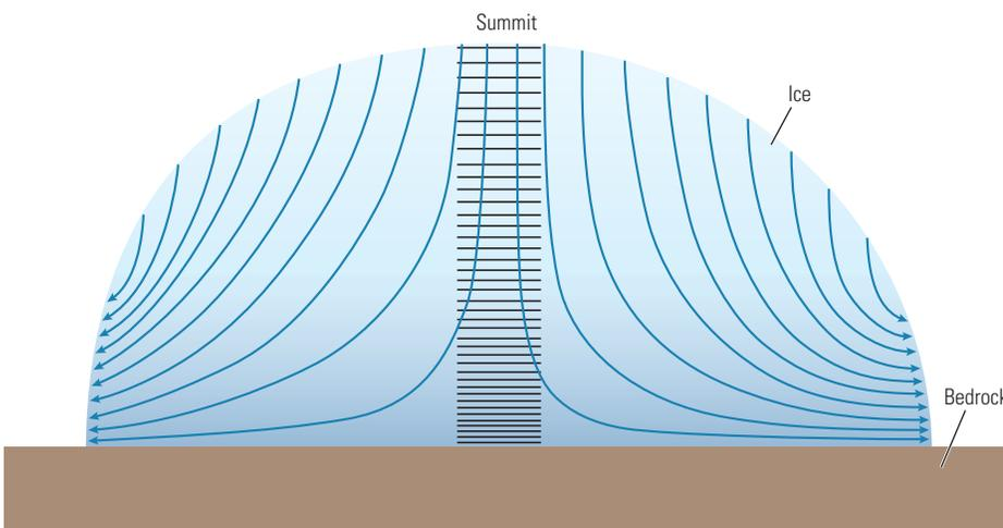
▲ Ice flow. Because ice is plastic, it flows downward and outward (blue arrows) from the summit of a dome. Therefore, ice cores taken from the center of a dome (horizontal black lines) retain a true depth-age correlation. The black lines represent layers that become thinner with depth as they are compressed by increasing overburden weight.
