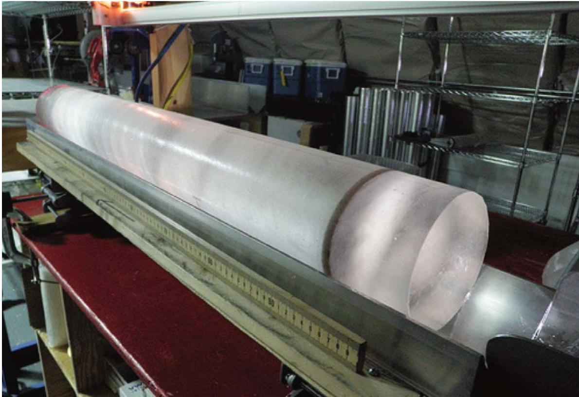
▲ West Antarctic Ice Sheet core. Because snowfall at the WAIS Divide rarely melts, ice layers for the past 40,000 years are unbroken, and their divisions are visible and easily counted. The ice also contains much less dust than other ice sheets do. A dark ash layer, however, in this 2 m [6.5 ft] long core section is clearly visible. (Photograph courtesy of Heidi A. Roop, WAIS Divide Science Coordination Office, University of New Hampshire.)
