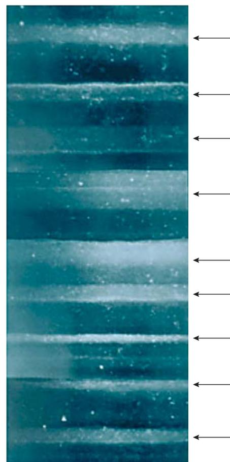
^ Visual stratigraphy. Annual layers are clearly visible in this ice core sample. Summer layers (arrows) appear lighter because they contain less dust. (Photograph courtesy of the University of Colorado Boulder, USA.)
