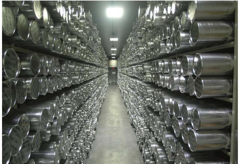
^ Cores in storage. The National Ice Core Laboratory in Denver serves as a center for preparation and storage of ice cores. The laboratory currently contains more than 17 km of ice cores from around the world.
