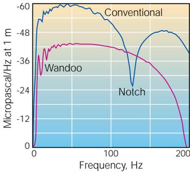
First, air guns were gathered into a tightly spaced array to act as a point source (*previous page, top*). The length of the gun arrays had to be reduced to match the overall shorter, denser sampling of the hydrophones. Concentrating the guns as a point source resulted in a more uniform wavefront (*above*). This contributed to producing a clean, high-frequency signature.
