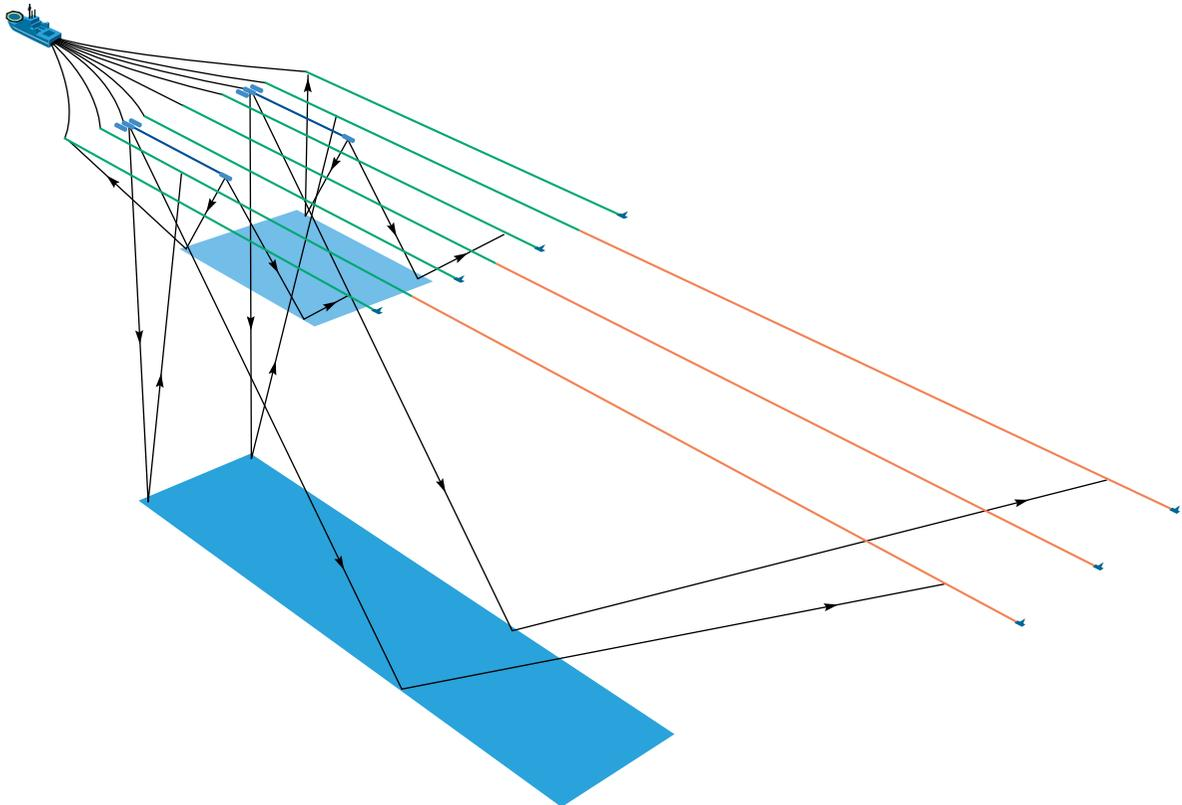
□A dual-purpose thin paintbrush and thick paintbrush. The multi-3D acquisition scheme can provide high-resolution images of a shallow target while simultaneously imaging a deeper target. The small shaded area depicts the zone investigated by the short streamer traces, and the large shaded area is that area investigated by the long streamer traces.
