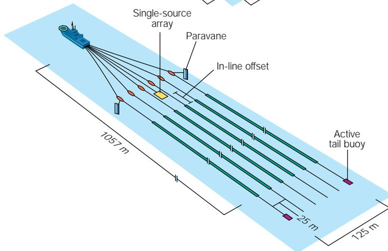
□ The Wandoo survey spread compared with a conventional spread (above). Streamers in the Wandoo survey (below) were 1057 m [3470 ft] long, about one-third the typical streamer length.
