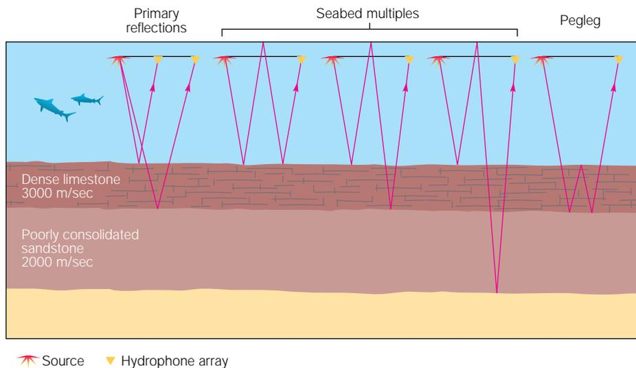
□ **Types of multiples in a marine setting.** In Wandoo, multiples tend to develop where a low-velocity layer overlays a high-velocity layer, such as at the interface of the sea and the limestone.
