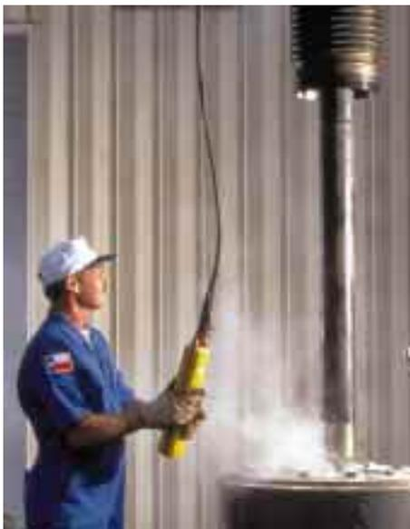
□ **New ultra-HPHT J-tools being pulled out of the test vessel after qualification testing.**
