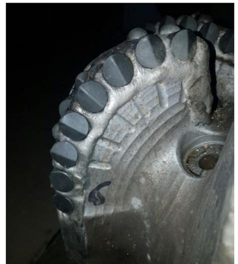
*Close-up images of undamaged AxeBlade bit cutting elements after drilling 365 m [1,197 ft] through a variety of challenging sections.*
