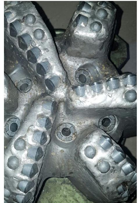
*Examination of the AxeBlade bit after pulling out of the hole revealed that it was in excellent condition and rated as rerunnable.*
