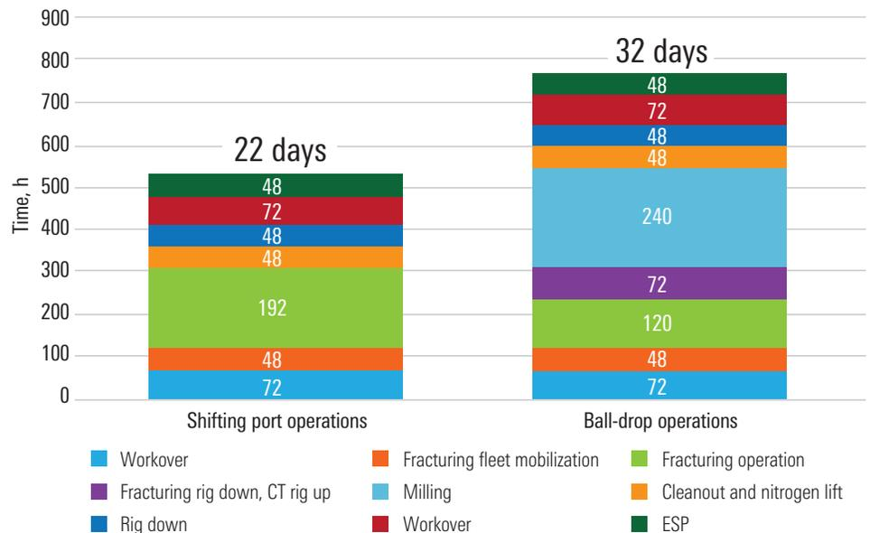
Completing 20 stages with coiled tubing and the sliding sleeve technology eliminated about 10 days of operations as compared with a ball-drop completion. Most of the savings is from eliminating milling operations.
