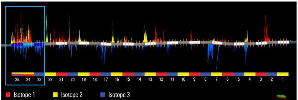
*The tracer log from the study well confirmed that Broadband Sequence fracturing service delivered 100% perforation coverage in intervals 23 to 25.*
