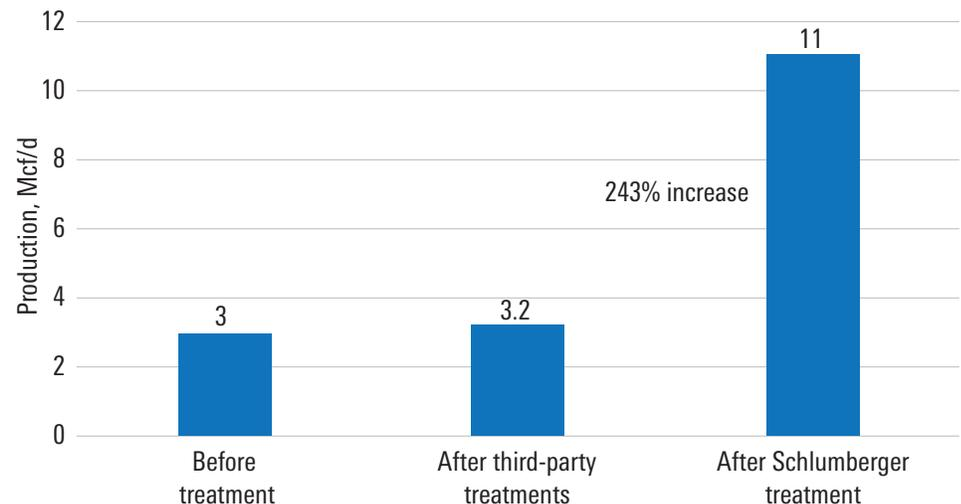
*Cleaning the perforations and stimulating with polymer-free VDA acid improved the well's production response by 243%—a significant increase compared with the small increment from previous third-party treatments.*
