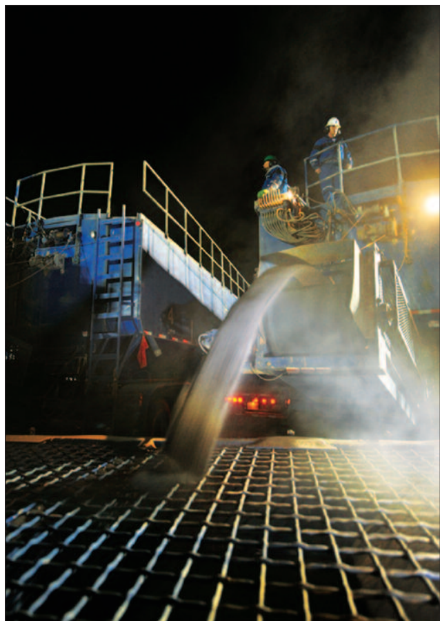
Field crews add ceramic proppant to a hydraulic fracture in the deep, hot Haynesville Formation. (Photo courtesy of CARBO)
