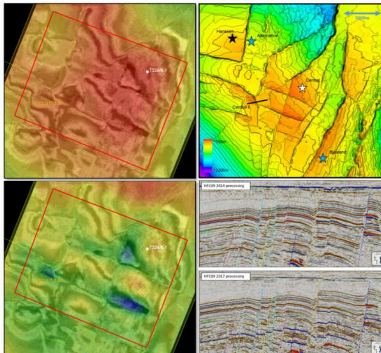
**Figure 3** Depth slice at reservoir level showing the FWI initial model (upper left panel), the final FWI velocity model (lower left panel), an illustration of the study area: The Wisting discovery in the Barents Sea (upper right panel). The lower right panel shows the image improvements after the reprocessing and model building workflow application. Upper seismic section shows the legacy PSTM image and the lower section shows the reprocessed data.
